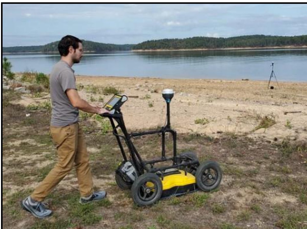
Figure 2: The GPR and GPS systems deployed on site, as shown in a stock photo from Bigman Geophysical.
